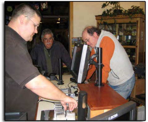
Tim Gibson from Weights and Measures looks on as the scales are being calibrated.
